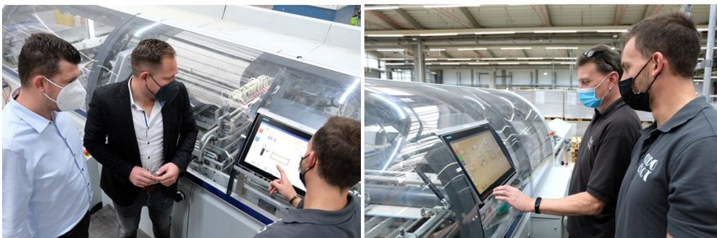
*To meet production demands at Ludo Fact, Kolbus developed a new machine configuration linking two DA 290 inline casemakers complete with automated pallet feed and output stacking.*
